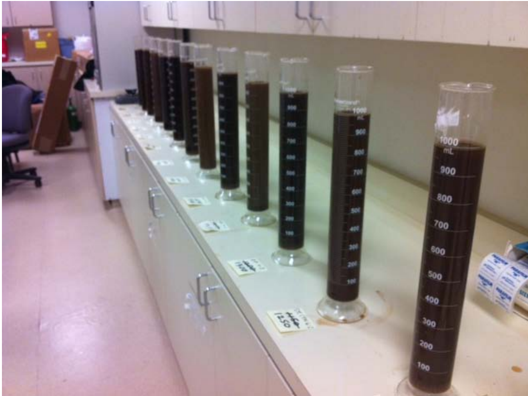
Figure 16. Soil solutions in graduated cylinders await measurements as sediment settles over a period of 3 hours. Relative density measurements are taken using a hydrometer at 40 seconds, 2 hours, and 3 hours after mixing.
