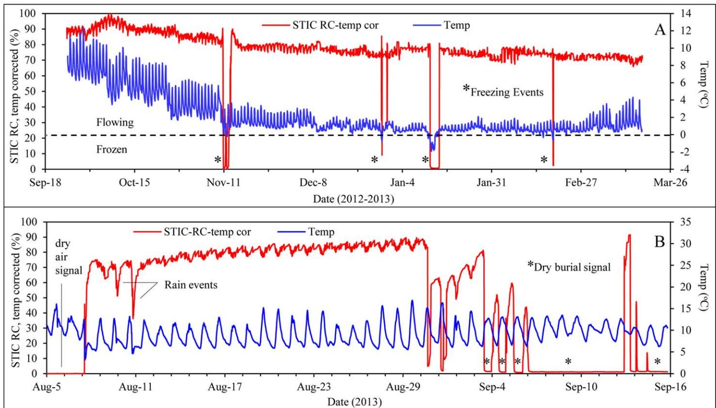
**Figure 3.** Seven month overwinter STIC deployment in the thalweg of Trinchera Creek, CO (a). Frozen conditions and flow cessation were recorded 4 times during the winter. The ice RC signal was 0.5% and distinguishable from an air signal (RC=0). The effects of sediment burial with diel wet-dry cycles in Cat Creek, CO (b). Note that the RC dry signal was 1% and not an air signal (RC=0) and temperature data alone did not indicate multiple dry-wet events in Figure 3b.
