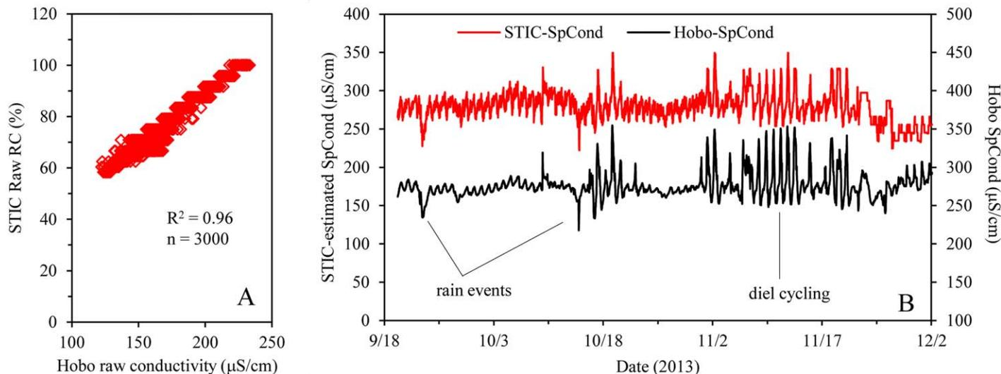
**Figure 4.** Comparison of raw STIC RC data and raw conductivity data from an Onset conductivity logger (a). Comparison of STIC estimated specific conductivity versus specific conductivity measured by Onset HOB0 conductivity logger (b, note y axis scale offset to separate data). Rain events and diel conductivity cycling were captured by both instruments.
