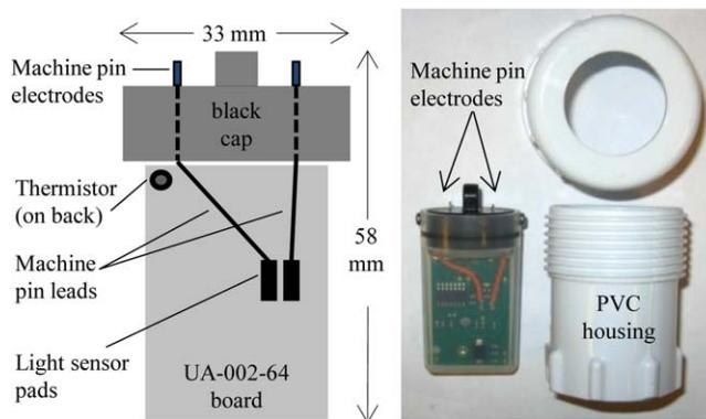
**Figure 1.** STIC electronics modifications and PVC deployment housing. The STIC can be concealed with rocks if vandalism is a concern.
