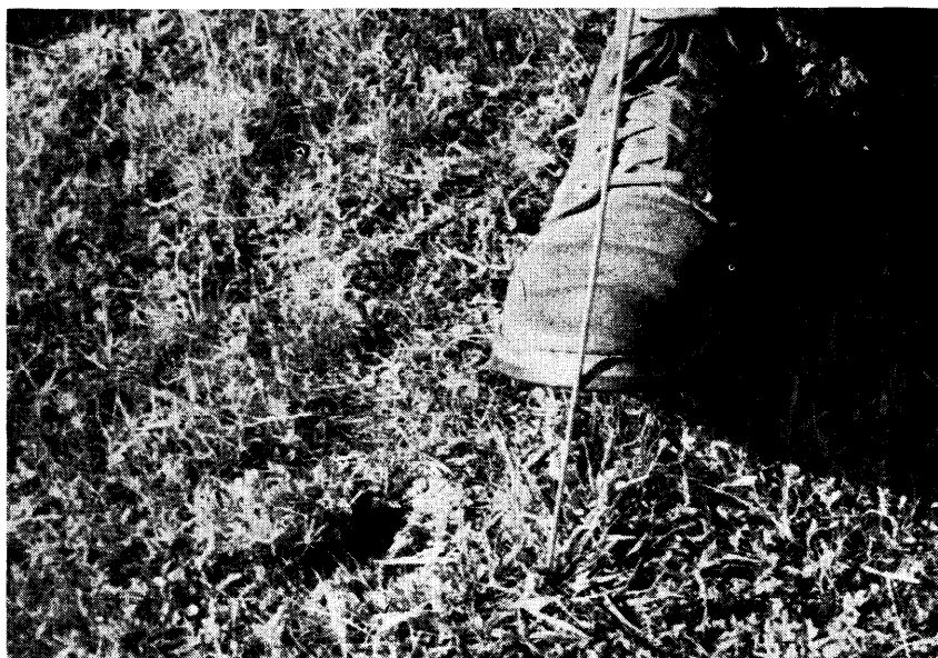
FIGURE 1. The sampler is establishing a sampling point with the use of a pin and a notch on the toe of his boot—the step-point.
