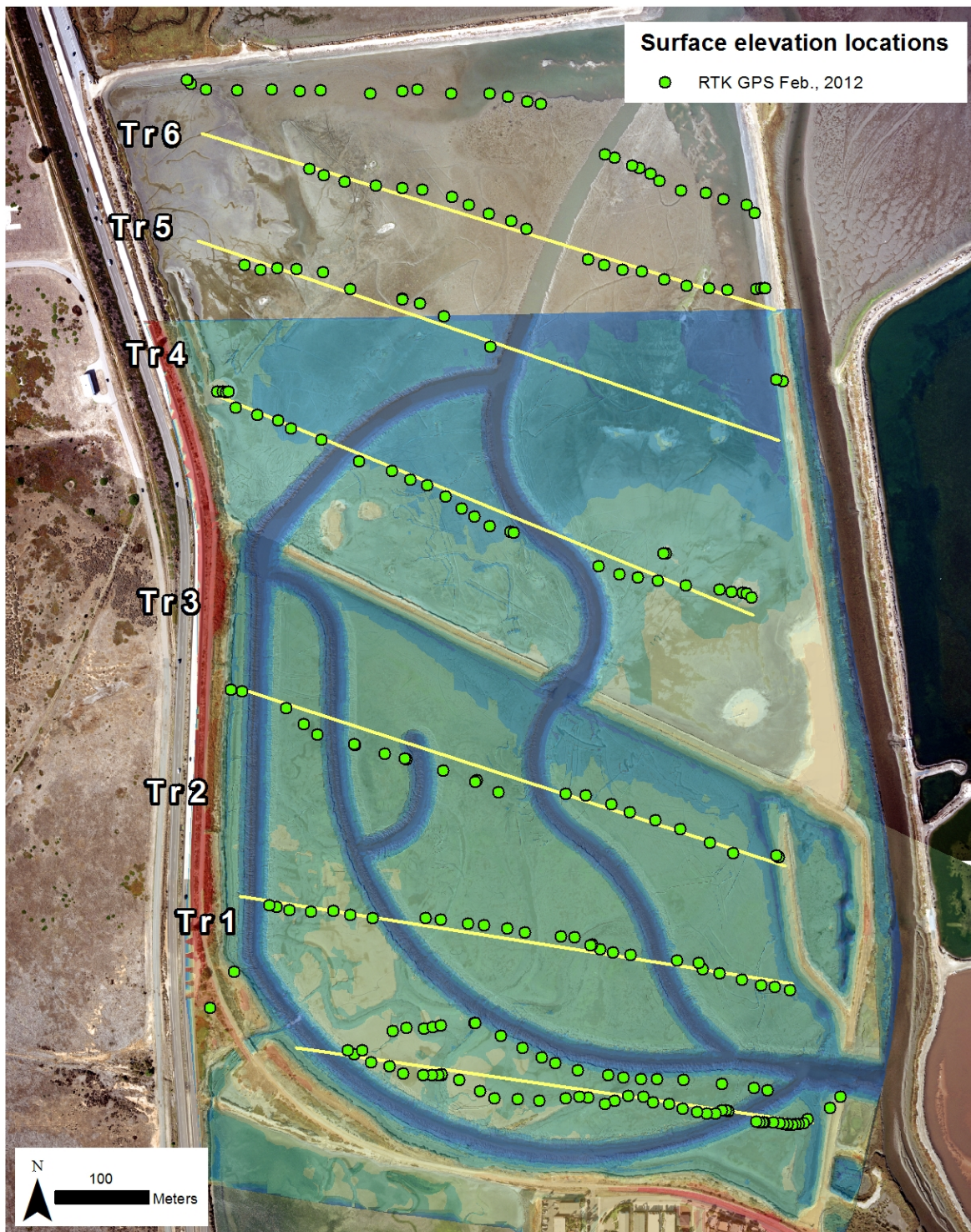
Figure 3. Real Time Kinematics Transects and Data Points Taken for Marsh Plain Topography February 2013.
