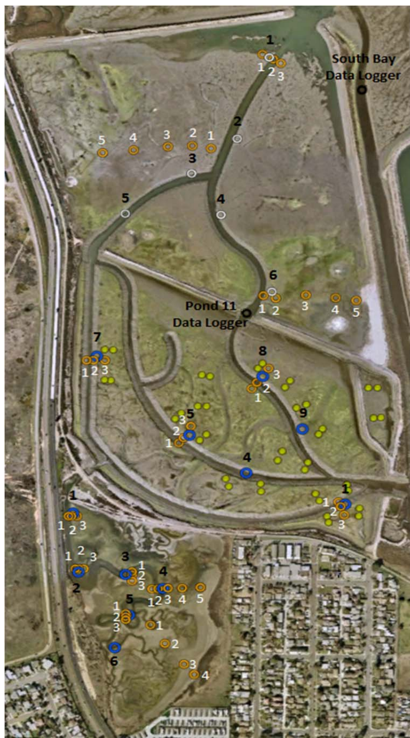
Figure 7. Monitoring Stations Western Salt Ponds. Locations of water quality data-loggers are shown in black. Green dots = corners of experimental vegetation plots. Blue circles = enclosure traps and invertebrates. White circles = invertebrates only, both channel-bottom and tidal flat. Brown circles = sediment.
