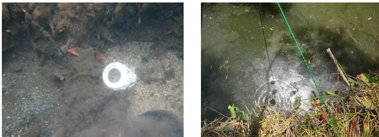
Figure C5. Showing various STIC locations, anchoring techniques, and visibility. (From top to bottom, left to right) 1. Anchored with spray-painted rectangular stake, 2. Visible in sandy stream channel, flagged, 3. and 4. Hidden under large rock, 5. Underwater, and 6. Anchored to tree with a cable.
