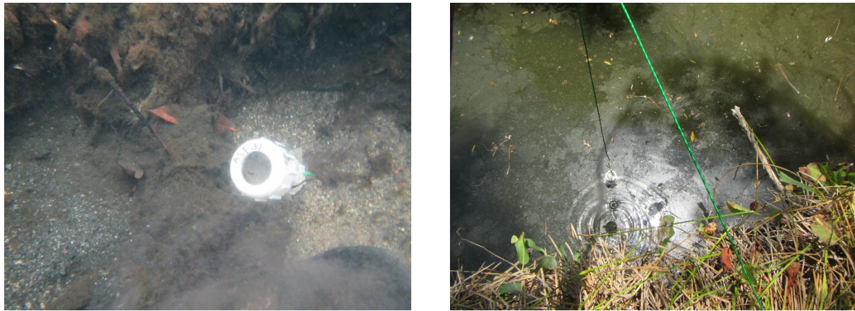
Figure 3. Showing various STIC locations, anchoring techniques, and visibility. (From top to bottom, left to right) 1. Anchored with spray-painted rectangular stake, 2. Visible in sandy stream channel, flagged, 3. and 4. Hidden under large rock, 5. Underwater, and 6. Anchored to tree with a cable.
