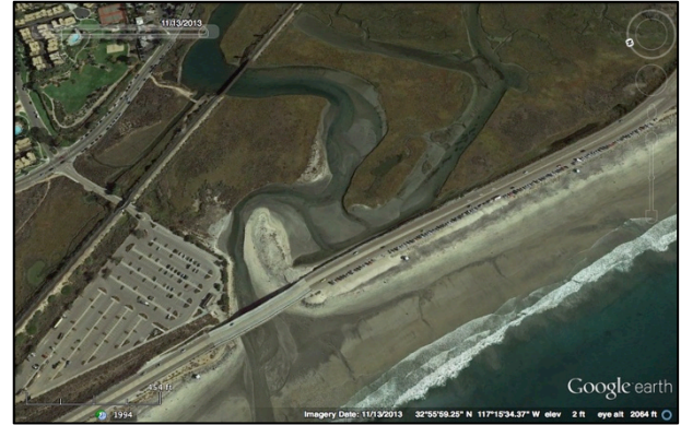
Figure 47. Inlet at Los Peñasquitos Lagoon in 2013. Note the almost complete loss of the remnant dune system as the main channel shifts to the northeast. Google Earth.
