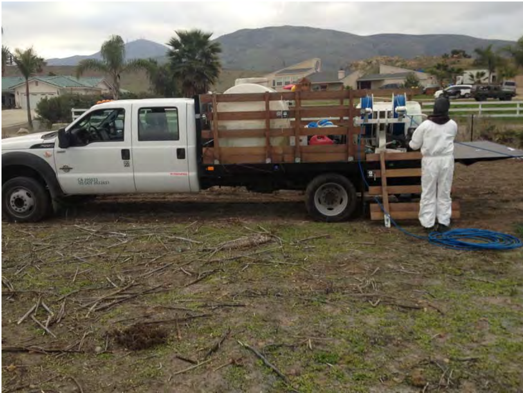
Photograph A.1. Truck-mounted reel-spray rig.
